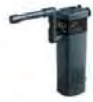
Model HL-BT100 8W VOLTAGE: 110-120/220-240V FREQUENCY: 50/60Hz FLOW: 150L/h MAX JET: 0.5M SIZE: 43x37x31mm
